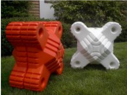
A standard module weighs 36 lbs. Empty, and is approx. 30" X 30" and 22" deep. The module can be filled with materials of different densities, such as water or sand, to precisely adjust its buoyancy as well as provide ballast. The modules can also be "puncture proofed" by filling them with marine buoyant foam. The modules can be produced in any color, and come standard in white, black, and a highly visible safety orange.
